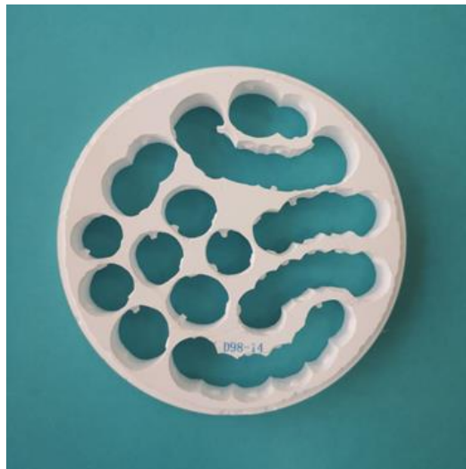
Figure 3.1: CAD/CAM machined pre-sintered zirconia block
